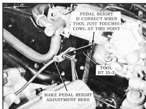
Fig. 8-126 Checking Pedal Height
