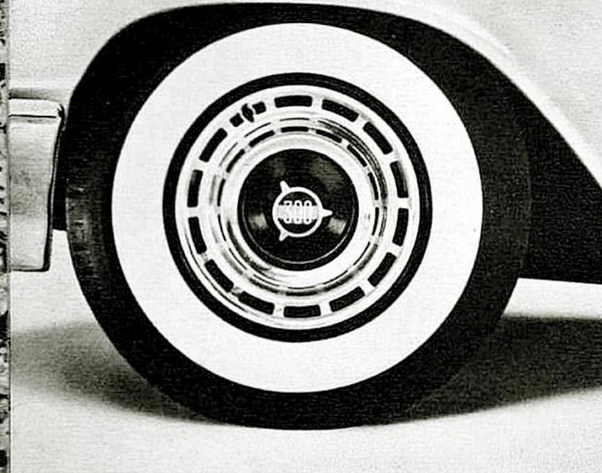
New 15-inch wheels, fitted with sports-tread tires and ventilated wheel covers, greatly improve brake cooling . . . cut brake fading.
