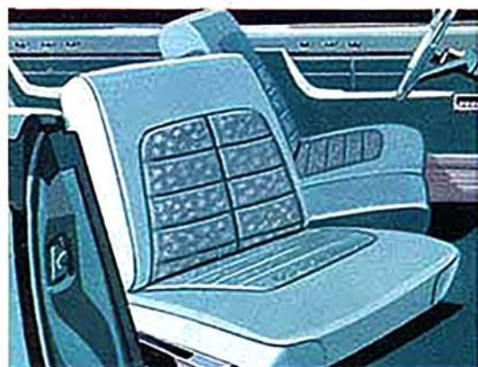
Automatic Swivel Seat swings out as you open the door—swings in when you leave the car. A moderately priced Chrysler option.
