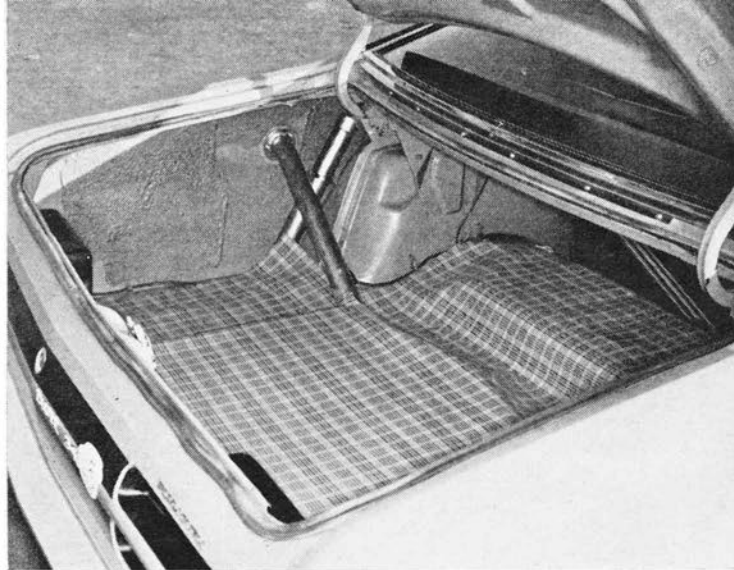
BIG TRUNK has spare hidden under the floor. Second tube under fender is vapor separator for smog control.
