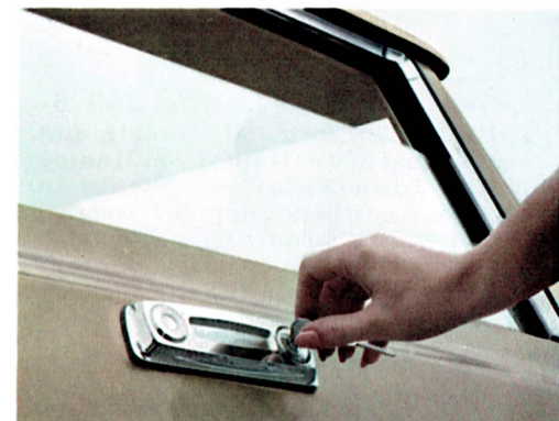
Power gate window has dual controls.
