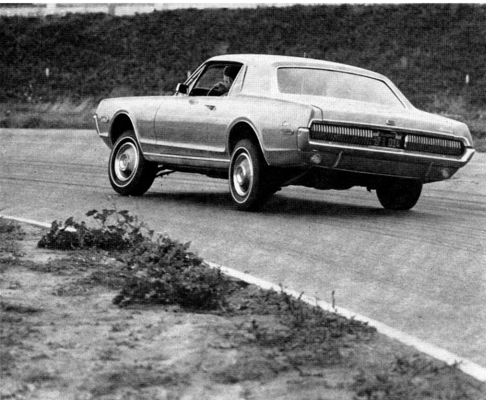
EXTREME LIFT of inside of standard Cougar occurred at relatively low cornering speeds. Inside front tire shows alarming camber angle, with only inner edge of tire maintaining contact with pavement.
