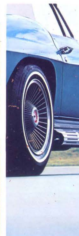
Whitewall tires and dual side-mounted off-road exhausts
