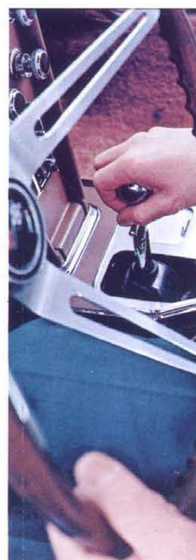
Console-mounted 4-Speed shift lever
