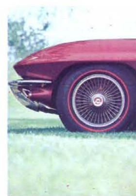
Red-stripe tires and special cast-aluminum wheels
