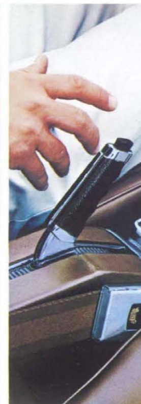
New console-mounted hand brake lever
