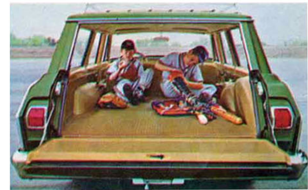
Nova Station Wagon Interior in saddle, offering 76 cubic feet of cargo space. Covered spare tire and wheel are conveniently carried upright in right rear quarter panel wall.
