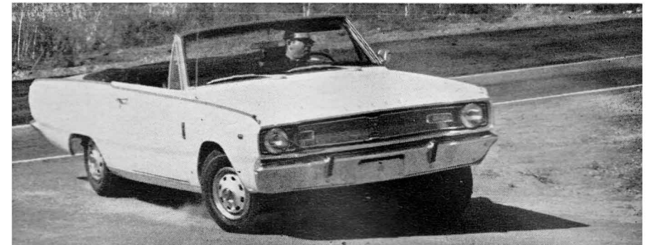
Heavy-duty rear springs, front torsions bars, sway bar and disc brakes, are part of Dart's Rallye Package, do wonders for its safety and handling as seen here.
