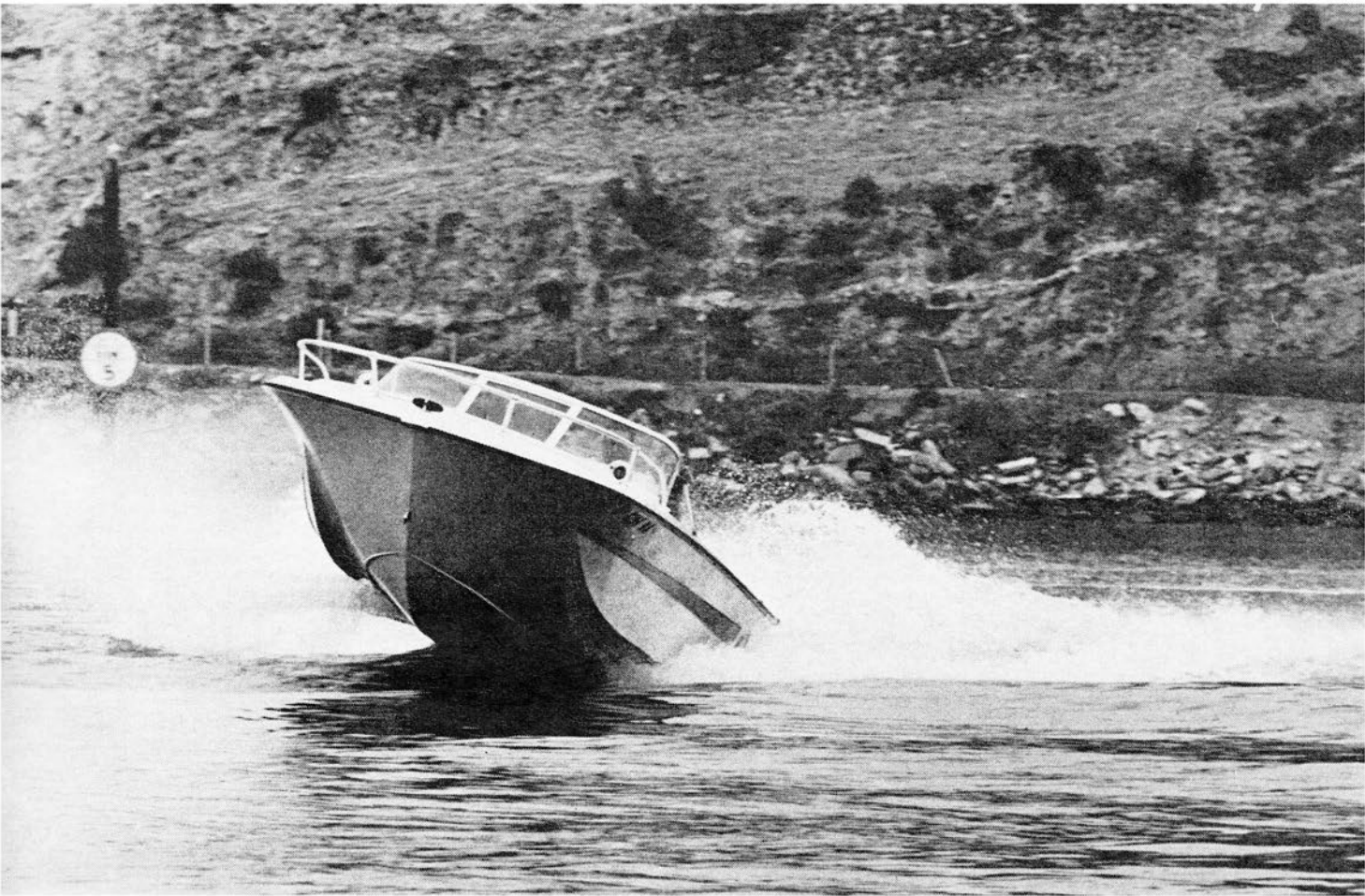
HYDRO-VEE design aims to provide stability when the boat is at rest, when moving slowly and at brisk speeds through turns. The Courier 229 Model, above, is capable of an estimated 30 mph at 3000 rpm from the 225-cu. in./150-bhp Slant Six.
