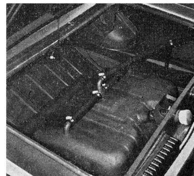
37-gallon fuel tank is assured of ambient pressure by this extra-large vent.
