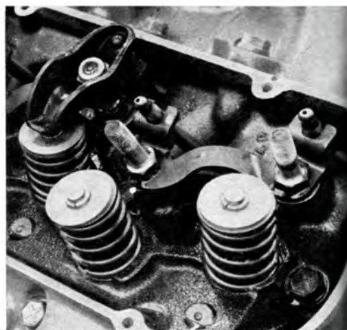
ABOVE—The unique rocker arm configuration incorporates the stamped steel guides to control push rod motion. Splayed valve arrangement is reflected by stem angle. Rocker studs screw in.
