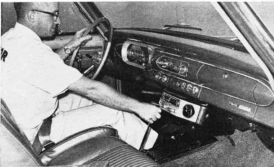
Dash of SS model is simple, easy to read, and uses gauges instead of warning lights. Automatic shift lever is vague in operation. Protruding knobs could bark knuckles.
