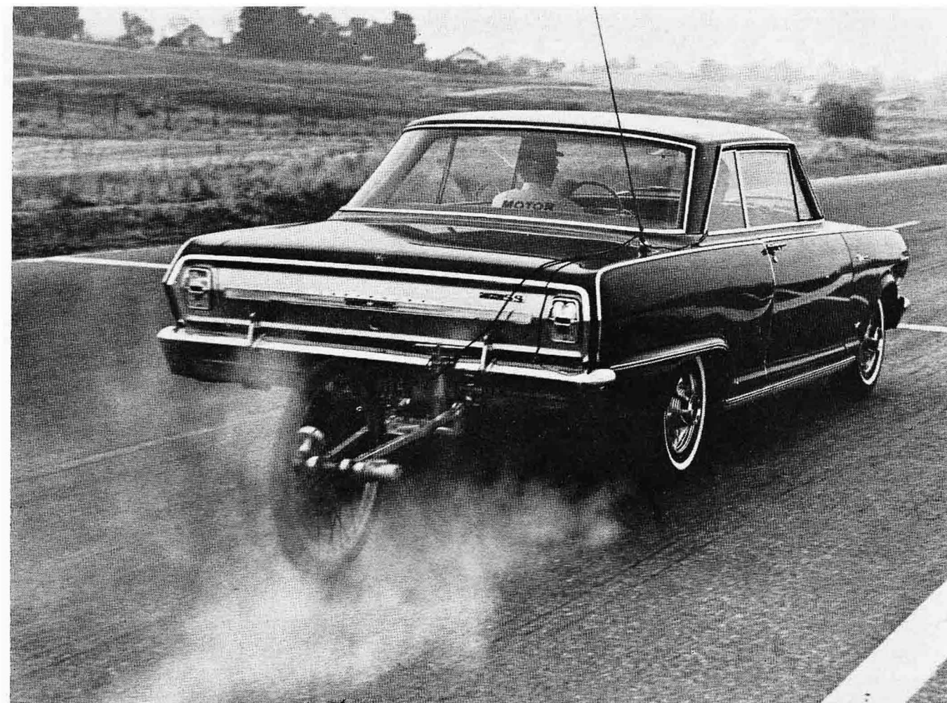
ALTHOUGH CAR DOESN'T HAVE OUTSTANDING STOPPING POWER, BIGGER BRAKES SHORTENED LAST YEAR'S BRAKING DISTANCES BY 30 FEET.
