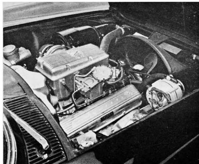
LARGE AIR-collector box dominates top of only fuel-injected engine in an American car.
