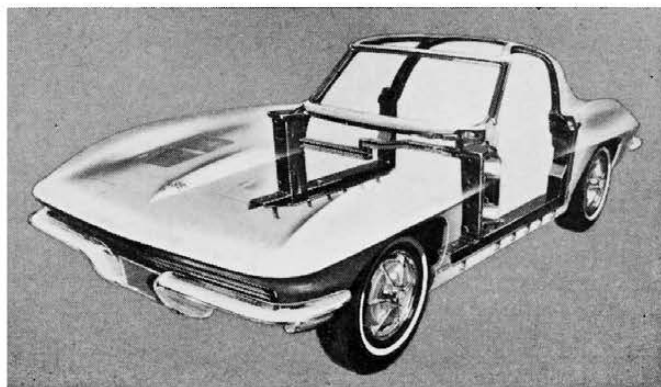
STEEL STRUCTURE is used as reinforcement for fiberglass body around cockpit area. Rubber body mounts have been changed.
