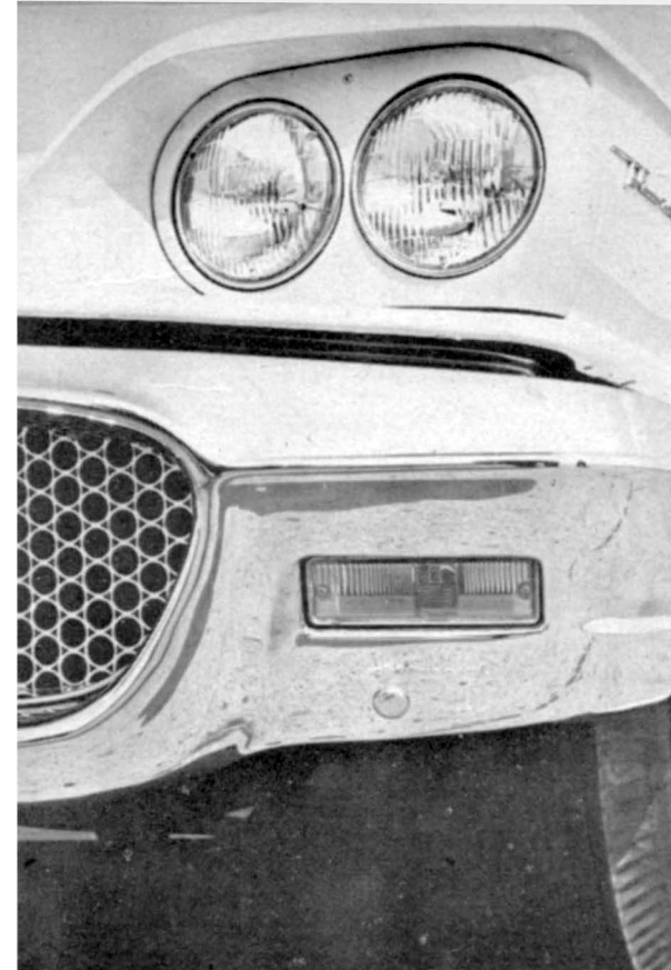
Front is blunt looking, with four headlights set in fenders; riding lights and grille in bumper.
