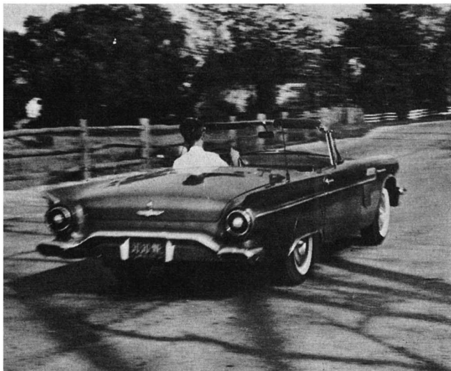
Driving position is generally good, and bench-type seat gives fair lateral support. Low steering wheel makes entry awkward for a long-legged driver.
