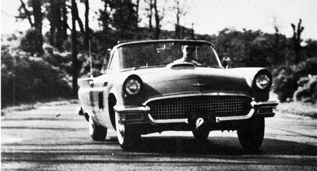
Car leans badly going into a fast turn, although it feels fairly flat to driver. With more than four turns lock to lock, on tight bends car becomes quite a handful. Power assist is excellent on the T'Bird.
