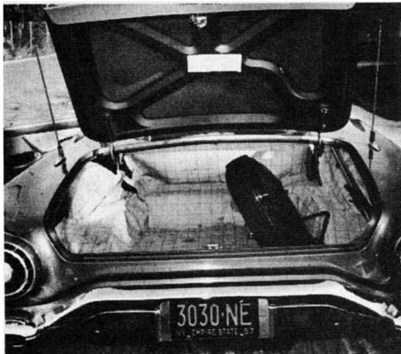
Angle of spare tire keeps trunk deck low, but cuts space available for luggage storage.
