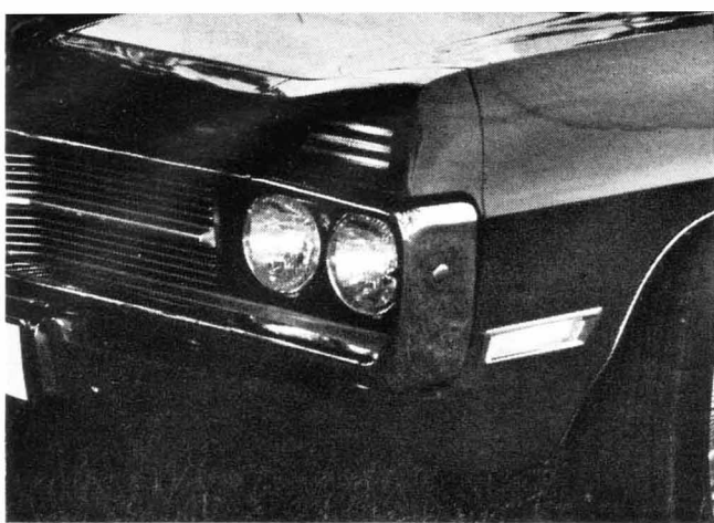
Grille section flips out of the way, exposing headlights. Note eyebrow-hooded parking light, above. Turning lights are options.
