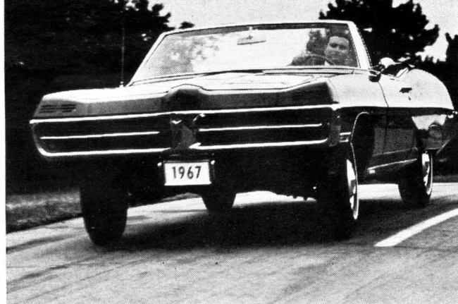
The big Grand Prix was amazingly stable when driven hard. Note left front wheel off the ground as it tops a rise at speed.
