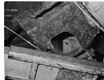
Above, welded-in torque boxes were used to support roll cage. Below, stock street hemi rear suspension is very similar to last year's factory race car setup.
