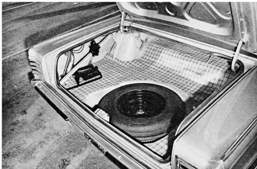
SPARE TIRE fits inside trunk well, leaving broad, nearly flat area for carrying luggage. Jack components are tied down by a spring to keep them from rattling.
