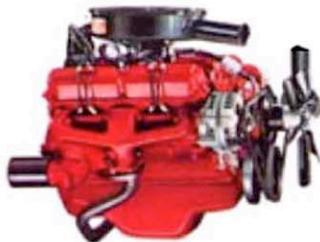
Husky 273-cu.-in. V-8 engine develops 180 hp at 4200 rpm.
