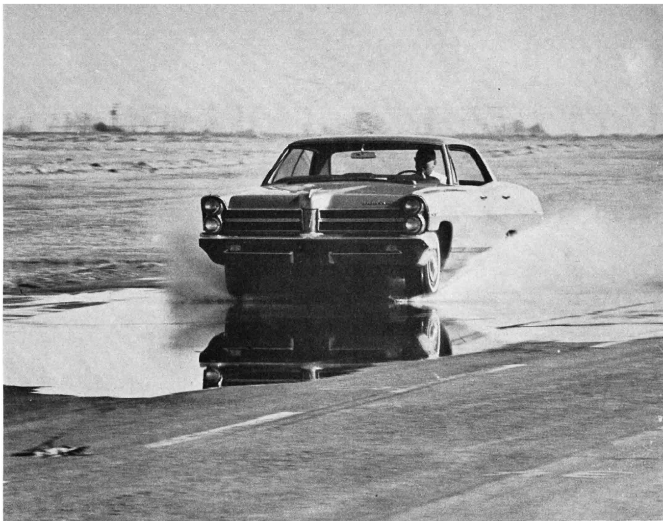
BLASTING THROUGH DEEP PUDDLES FAILED TO AFFECT CAR'S BRAKES OR DIVERT ITS COURSE. STOPPING WAS ALWAYS STRAIGHT AND TRUE.
