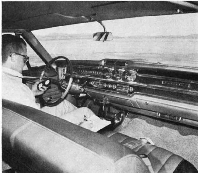
Three round gauges—one a clock—are angled in toward driver for easy reading. Front and rear vision put all fenders in view. Test stopwatches clocked Catalina's strong acceleration.
