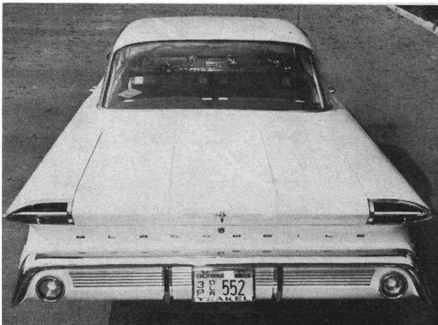
The rear window on hardtop '60 models features heat resistant glass. Upper portion of the glass is "aluminized" to reflect heat but when the sun is high overhead, it acts somewhat like a mirror; driver sees reflections when using rear view mirror.
