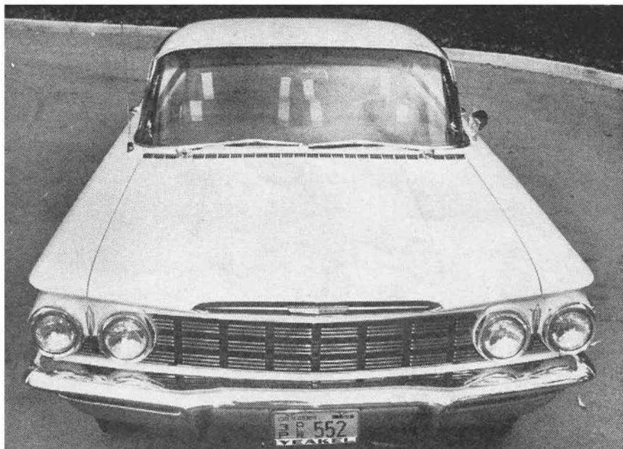
Oldsmobile's 1960 body is 80.6 inches wide and the broad expanse of sheet metal in front of the windshield is hard to see over. Parking in close quarters is usually a matter of guesswork because it's impossible to see right front fender from driver's seat.
