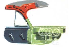
Armor-rib body construction is a worthy match for Packard's husky chassis construction. The solid thud you hear, when you close a Packard door, is quick evidence of this body's immunity to twists, rattles, and outside noise.
