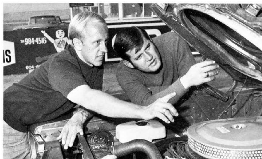
At Press Day showing, Ronnie Sox, left, and CC Associate Editor Bob Swaim discuss the fine points of the Road Runner's "Coyote Duster" fresh air package. It's dash controlled.
