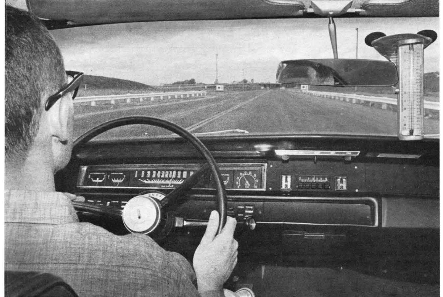
BRAKE TESTS from 80 mph, recorded by decelerometer on windshield, were disappointing. All-drum system faded and lacked balance.
