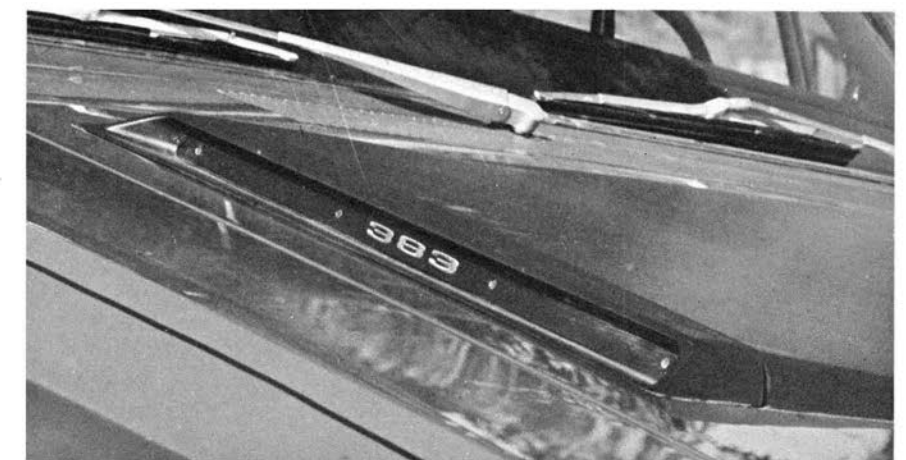
The two-foot-long hood scoop insert tells the displacement of the engine which is under the Road Runner's hood. Four screws can be removed to make the scoop functional.
