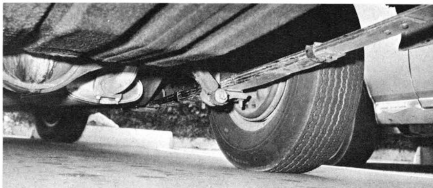
ABOVE: Suspension is heavy-duty type as are the shocks and brakes. A sway bar aids cornering which is a good feature of the car.
