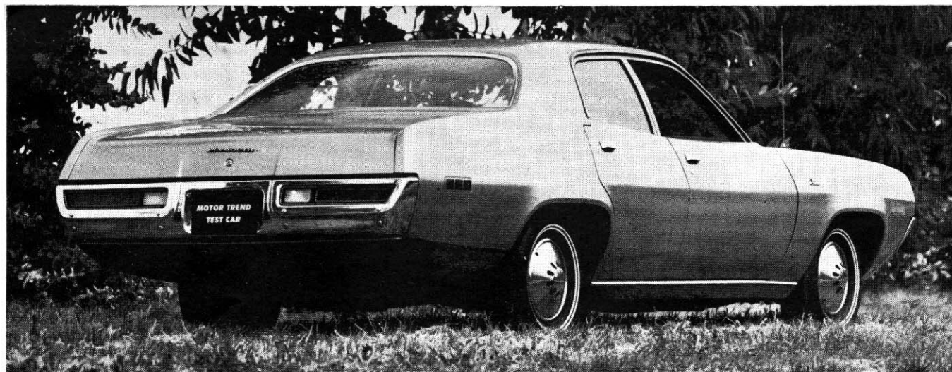
Above: Plymouth Satellite represents new Chrysler concept of designing four-door sedans with consideration for people packaging first, styling second. Result is a tastefully executed compromise with flared fender wells and upswept rear beltline to break the monotony of unadorned sheet metal. Horizontal taillights are placed, well protected, within bumper loops.
