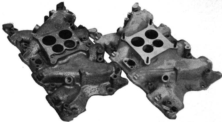
**ABOVE** — CJ and HO intake manifolds are identical in design, but the HO unit is cast from aluminum (right) while the CJ receives cast iron.
