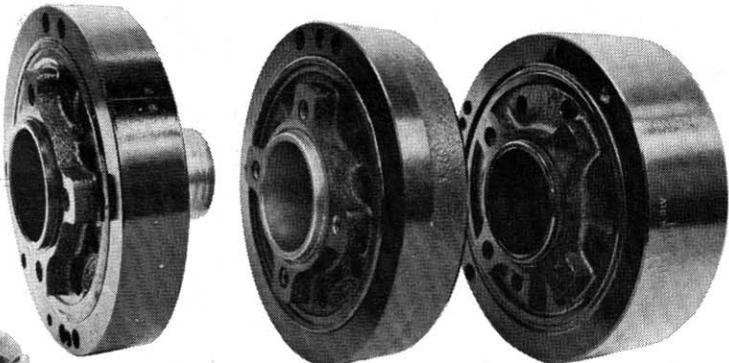
**ABOVE** — Harmonic dampers vary in weight for different engine applications. 2V and 4V engines get the lightest unit, while the CJ receives the middle-weight. The heavy damper is reserved for the HO.
