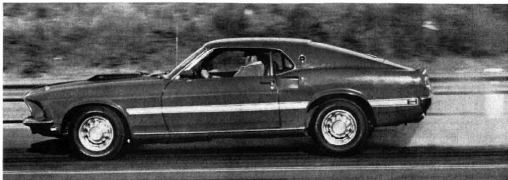
Mach I had accumulated several thousand miles by time of test, but brakes performed in excellent style. Both Mach I and Cougar brakes heated quickly, but neither ever faded.
