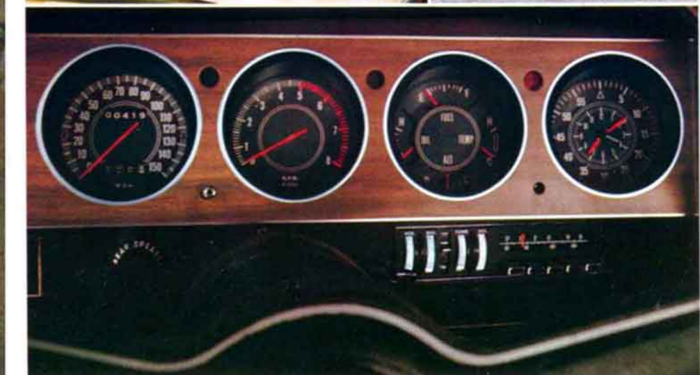
Nine-gauge lineup including trip odometer, tach, oil-pressure gauge, and clock.
