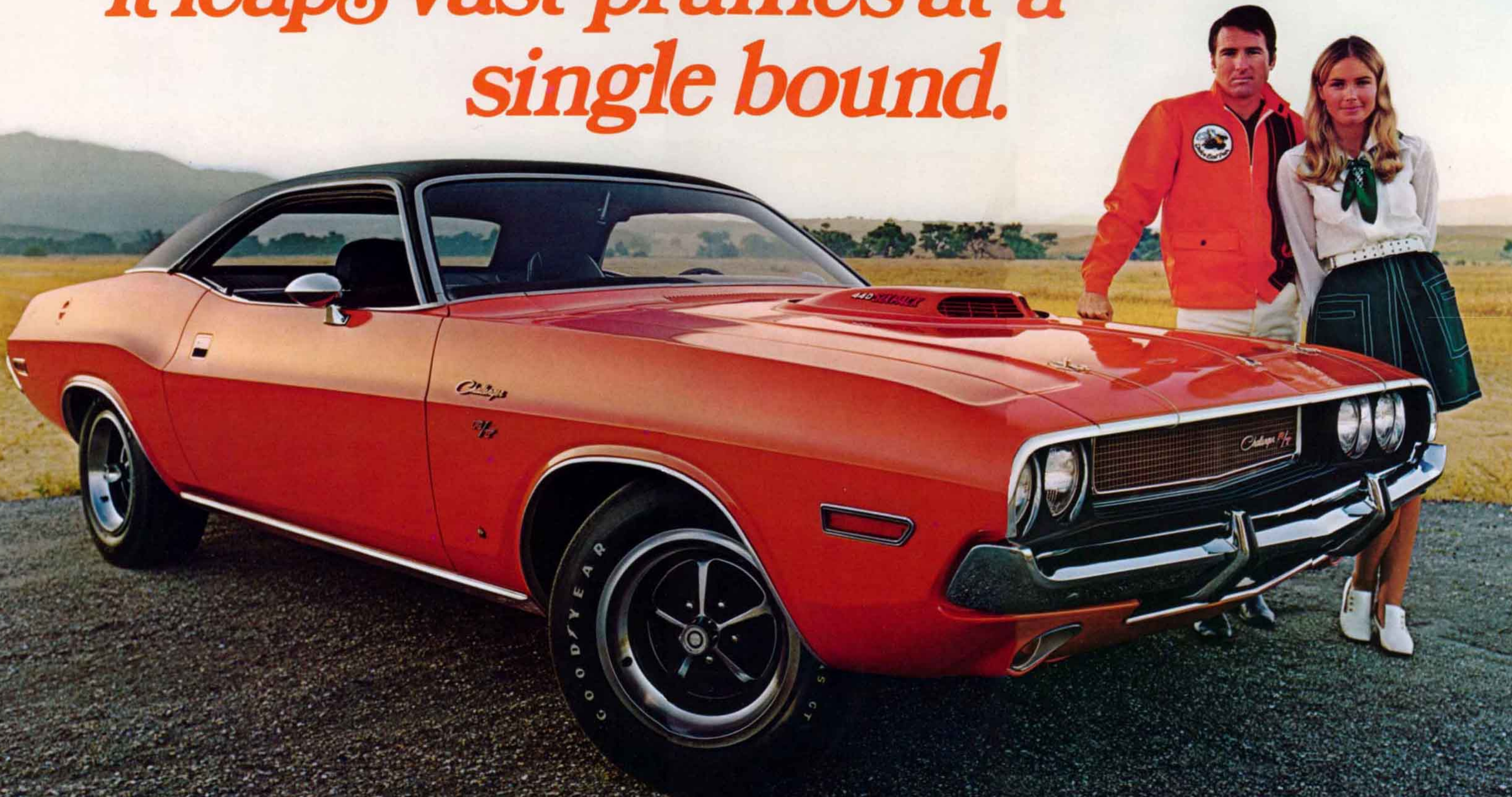
"Shaker" hood? Yes, functional scoop attached directly to carbs "shakes" at idle.
