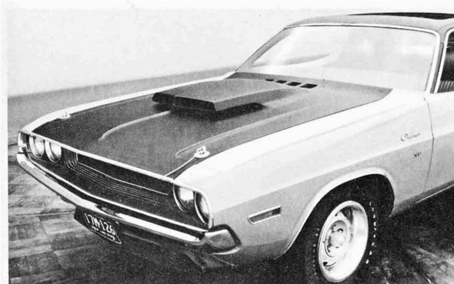
Black matte finished hood is a fiberglass job with special fresh air intake scoop.
