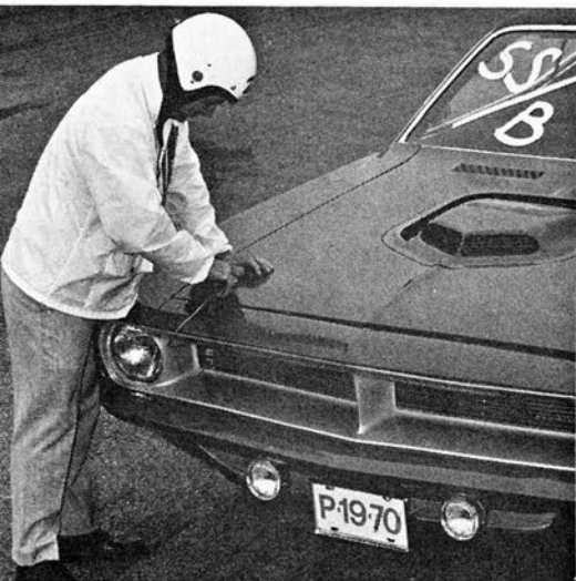
Hood pins are standard on the new 'Cuda along with the "Shaker" hood scoop with Hemi engine versions.
