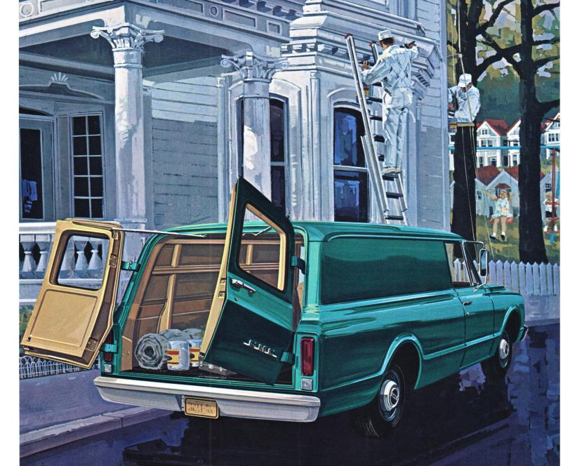
Rear lift and tailgate is offered in Suburban models for those who prefer station-wagon-type rear doors. The tailgate is flush with floor when open, permitting you to carry longer loads safely. Loading is easier, too. The liftgate swings up and out of the way for loading bulky, hard-to-handle cargo.
