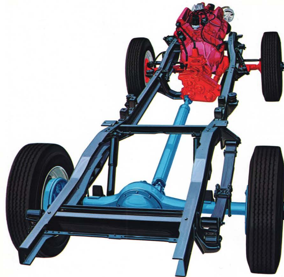
Front driving axle joints provide firm, positive power regardless of turning position. Forward-mounted steering gear and the high position of linkage protect mechanism in rugged terrain. Tapered leaf springs , front and rear,
