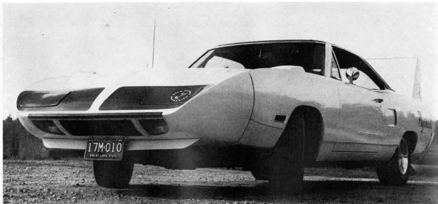
SuperBird differs from look-alike Daytona in more than location of air inlet, though concepts used in two were the same. Spoiler not only kills front end lift, but lowers overall drag by limiting airflow under car, and also aids engine cooling.
