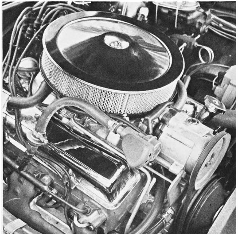
The high rev 302-cubic-inch Chevy features include a Holley four-barrel carburetor, high-winding mechanical lifters, special cam and aluminum inlet manifold.
