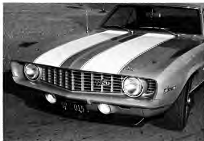
Front and rear spoilers are standard equipment on '69 Z/28 Camaros. These spoilers give Camaro much greater stability at high speeds.
