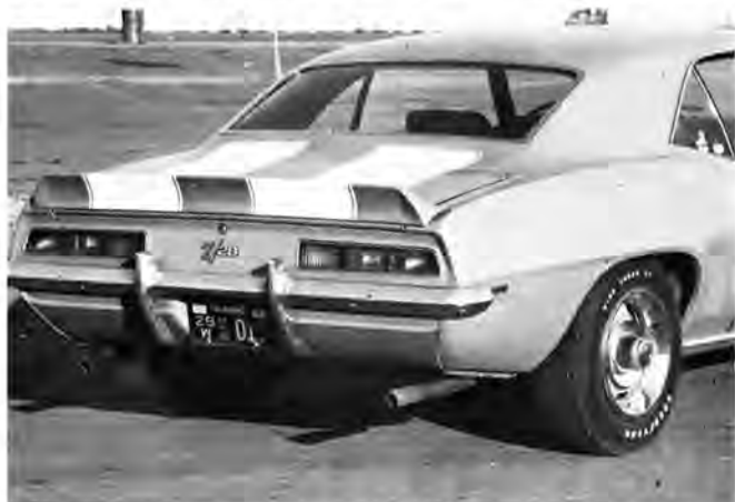
Front and rear spoilers are standard equipment on '69 Z/28 Camaros. These spoilers give Camaro much greater stability at high speeds.
