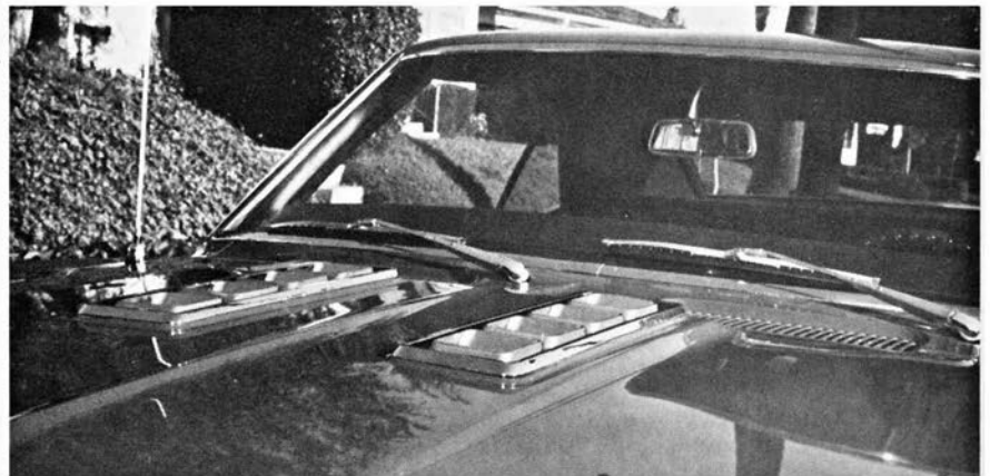
Dummy hood trim isn't functional, but is in keeping with sporty look of new Camaro.
