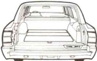
Dual Action tailgate is standard on all 1970 Dodge Coronet wagons.
