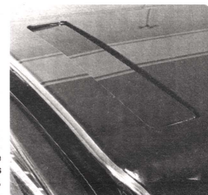
COLD AIR is controlled by engine vacuum. Cruising, near right, closes the door. Floor the pedal, far right, and the spring-load door pops open.
