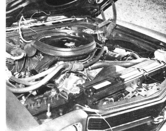
BULKY 396 engine is a tight fit. Soft rubber lip atop air cleaner seals against the cold-air trap door in hood.
