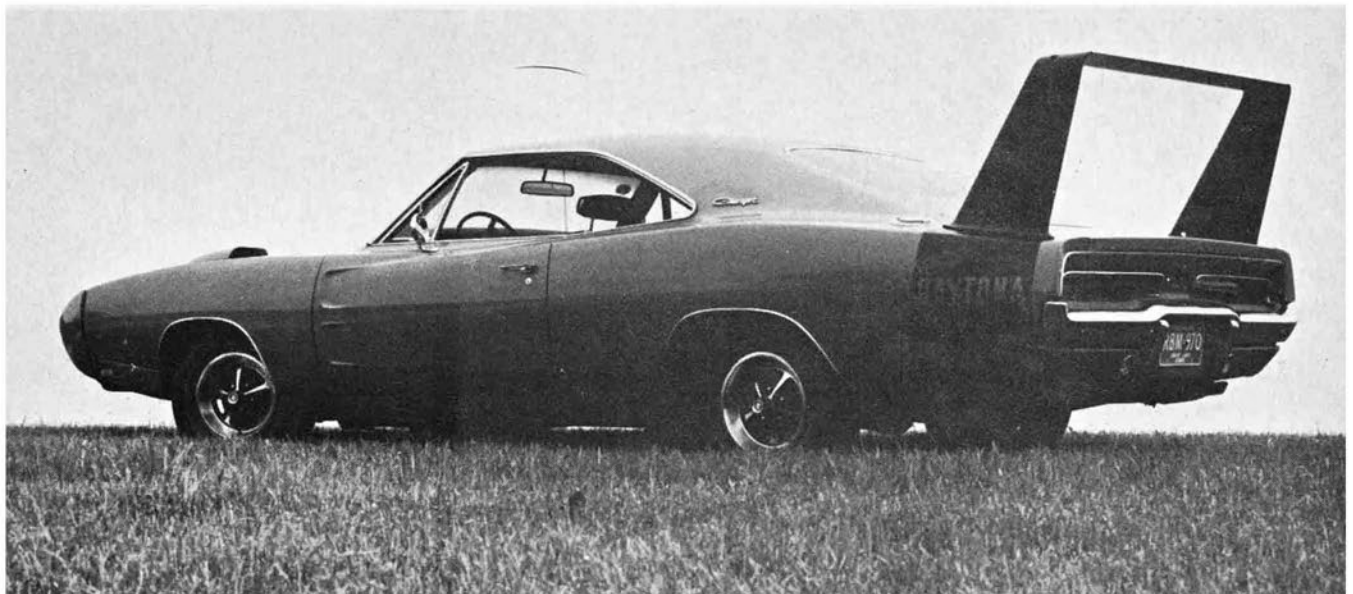
Charger 500 fastback roof and extended wedge front account for a 15 percent fuel economy increase at 70 mph over conventional Charger.
