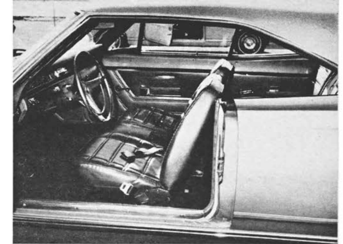
PLYMOUTH seats rated highest with testers—semi-buckets moved independently; center folded down for third person.
