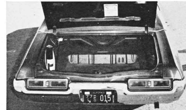
COLLAPSED spare in Pontiac turned the smallest trunk into car with most usable trunk space. Wheel tucks under fender.
