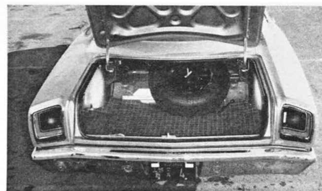
REAR mount for spare tire is also used by Plymouth, but Satellite lacked Ford's floor recess. Trunk lid was bigger.
