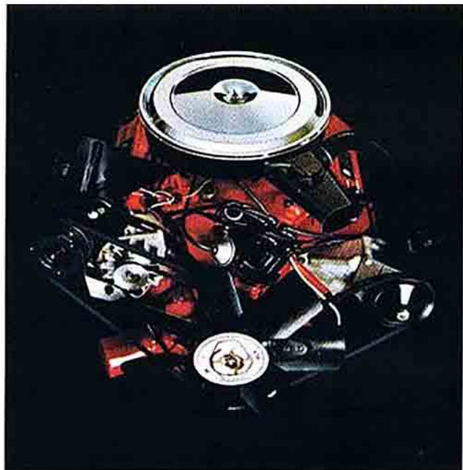
An entirely new engine for an entirely new automobile. The 350-4 V8. Standard equipment on the GS 350. 350 cubic inches. 4-barrel Quadrajel carburetion. Dual exhausts. Delivering 280 horsepower. 375 pounds feet of torque. The power you want. The dependable performance you want. And more economy than you'll believe.
