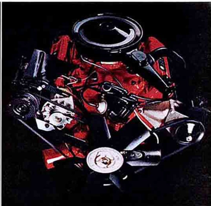
Another Buick powerplant that's new for '68. The 350-2 8-cylinder engine. 350 cubic inches. 230 horsepower. 350 pounds feet of torque. Power. Economy. Dependability. Standard on the Special Deluxe 2-Seat Wagon and all Skylark Custom models. Available on Special Deluxe Coupe and Sedans, Skylark Sport Coupe and Sedan.
