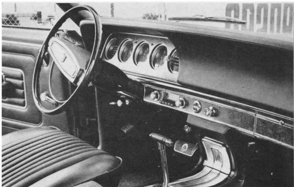
CYCLONE INTERIOR scored high marks for comfort and functionality. Instruments were readable, though lack of oil pressure and water temperature gauges with high-performance engine was discomforting and potentially dangerous.
