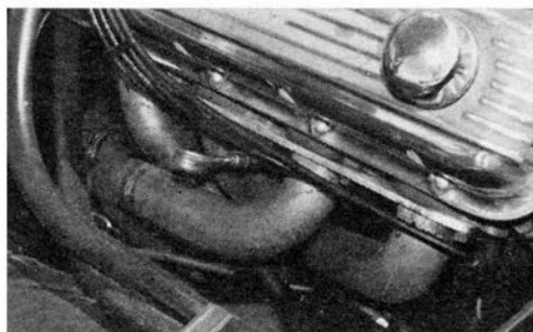
HEADERS nestle between engine and fender panels, help produce added power.
