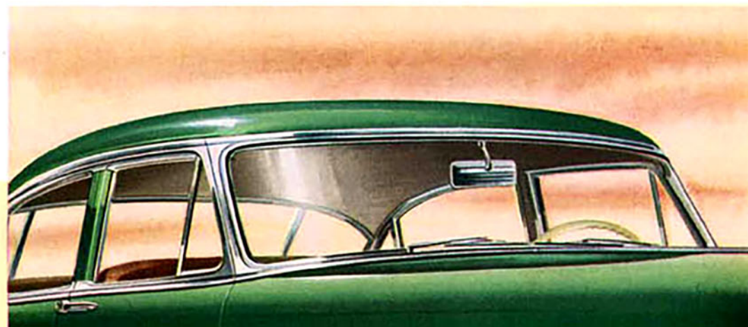
The large curved one-piece windshield with narrow corner pillars has more than 7 square feet of glass area. Cadillacs contain more than 3500 square inches of glass area.
