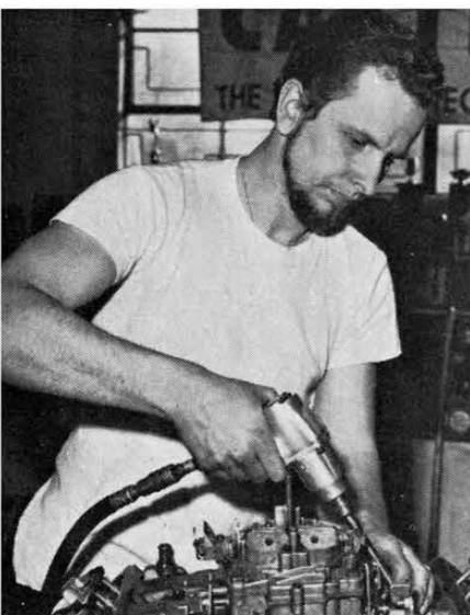
Boss Wrench Buddy Gromus tightens down manifold on 350 mill prior to GM test runs.
