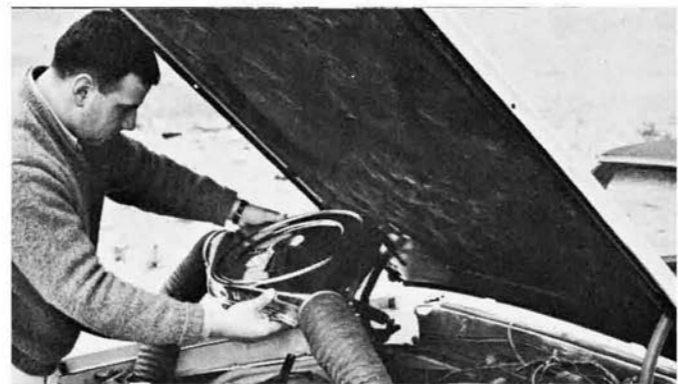
The cleaner lifts easily off Quadrajets when wing nut is removed.
