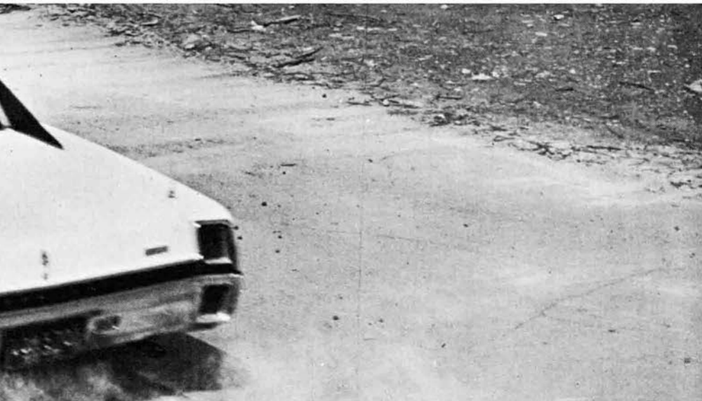
Wide Ovals bite nicely when coming off the line, but slicks would improve times.
