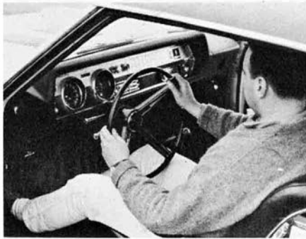
Adjustable steering wheel is operated by lever on the left side of the column.
