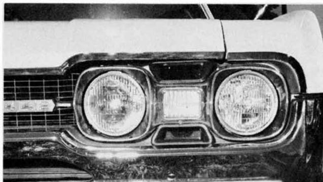
Located between headlights are fresh air scoops which are functional. Scoop outlets are attached by giant hoses to air cleaner.
