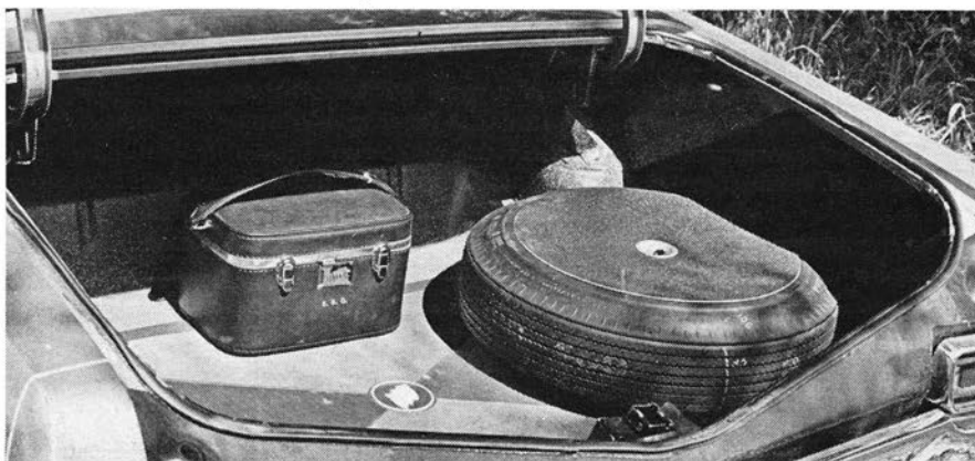
SIGNIFICANT PORTION of the large trunk volume is rendered inefficient by the intrusion of a floor mounted spare tire and wheel.
