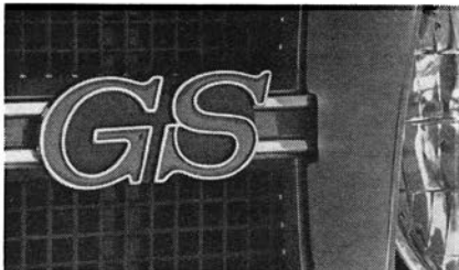
GS EMBLEM and dummy hood scoops add to the visual impact of the car, presenting a high-performance flair, while doing nothing for function.
